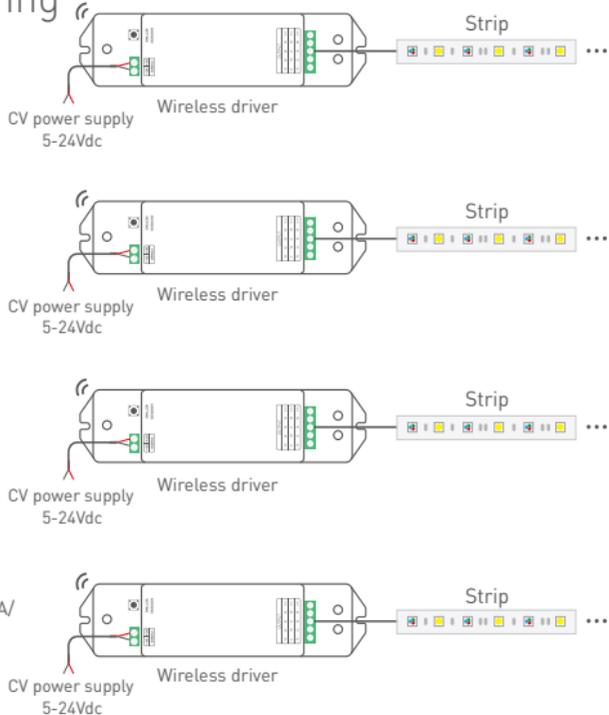
**To avoid the signal interference, the installation needs to keep away from the large area metal material or the metal material space.**
