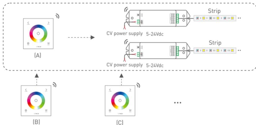
\* After touch panel A realizes controlling the lamps, if B and C are matched with A, they can also control the lamps.
