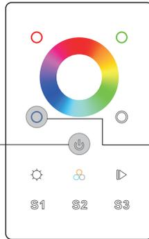
**Step 2:** Short press 5 times continuously to clear all bound lighting devices. LED indicator flashes 4 times for successful unbinding.
