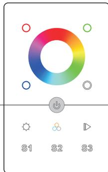
**Step 1:** Press and hold down until LED indicator turns on.
