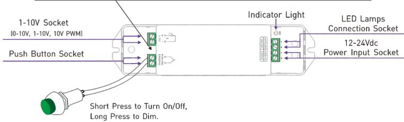
12V lamp connected, loads 0~144W(12V).
