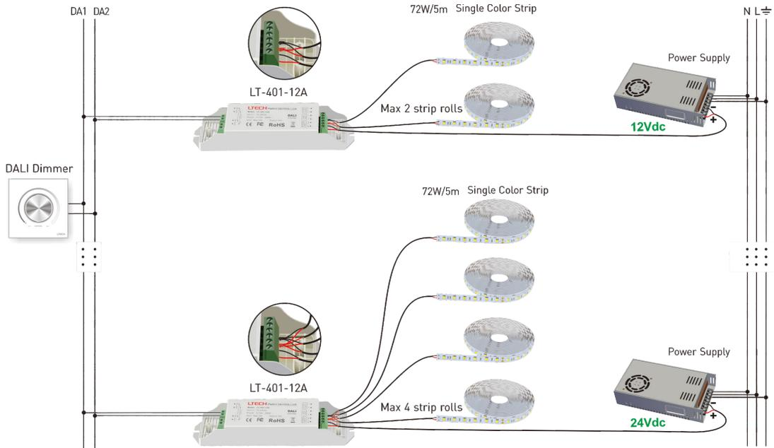
Providing DALI to 0-10V connect port, which is compatible to control 0-10V products in DALI control system, diagram example as below:
