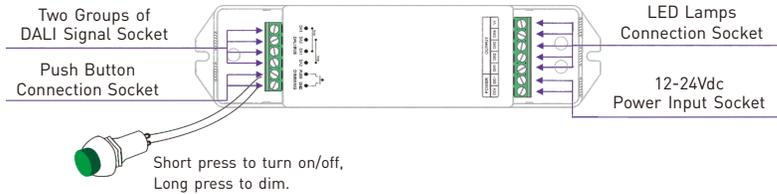
12V lamp connected, loads 0~240W(12V); 24V lamp connected, loads 0~480W(24V).
