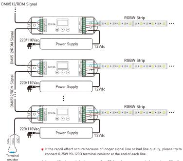
\* An amplifier is needed when more than 32 decoders are connected, signal amplification should not be more than 5 times continuously.
