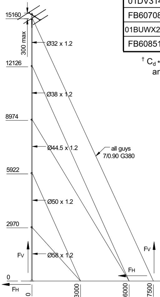
It is the responsibility of the installer to ensure that any structure to which the Telomast is fixed, as well as the fixing devices, are capable of supporting the design loads. The maximum ultimate limit state loads at the mast base and guy anchor points for the worst case loading situation are shown in the table above. The loadings are applicable to three and four way guying arrangements.
