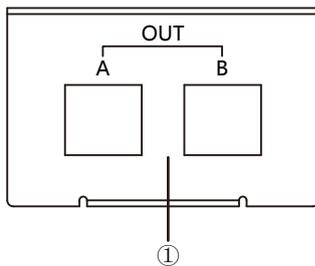
① TOSLink(Optical Fiber) Output Ports A and B: Connect the TOSLink output ports to the TOSLink input port of audio equipments such as audio amplifier and AV receiver.
