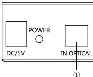
① TOSLink(Optical Fiber) Input Port: Connect the TOSLink input port to the TOSLink output port of audio equipment such as audio amplifier, AV receiver or DVD player.
