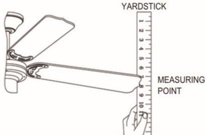
D/ Some fan movement is normal. However, interchanging an adjacent (side by side) blade pair may redistribute the weight and result in smoother operation.
