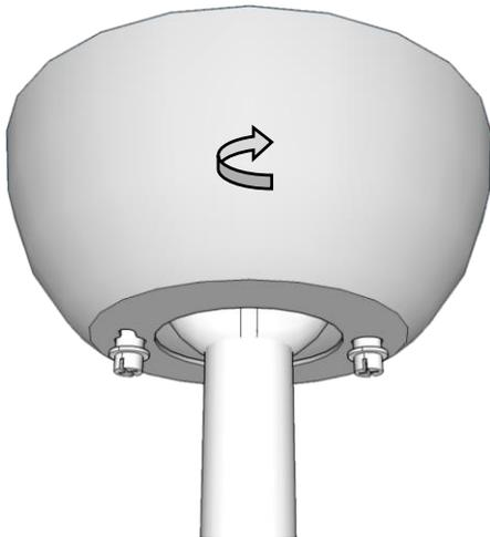
Carefully slide the canopy up to cover the hanging bracket and ball joint, taking care not to damage any wires. Once in position, secure the canopy with the screws provided.
