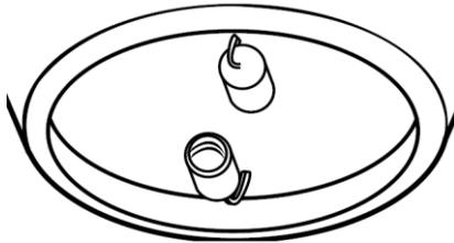
4. Attach the globes to the lamp-holders, make sure it is secure tightly.
