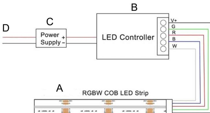
1. Connect COB LED strip light (A) to the LED controller (B).
