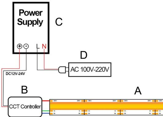
1. Connect COB LED strip light (A) to the LED controller (B).
