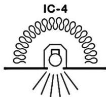
**A TYPE IC-4 RECESSED LUMINAIRE CAN BE ABUTTED AGAINST NORMALLY FLAMMABLE MATERIALS, INCLUDING BUILDING INSULATION, AND CAN BE COVERED IN NORMAL USE.**
