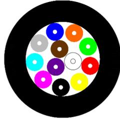
MaxCap BendBright® OM4 fibres are laser-optimised, bend-insensitive, graded-index multimode fibres engineered for transmission speeds of 10 Gb/s and higher. They are ideal for systems operating at wavelengths of 850 nm and 1300 nm. Featuring BendBright® technology, these fibres offer superior macro-bending performance.
