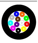
MaxCap BendBright® OM4 fibres are laser-optimised, bend-insensitive, graded-index multimode fibres engineered for transmission speeds of 10 Gb/s and higher. They are ideal for systems operating at wavelengths of 850 nm and 1300 nm. Featuring BendBright® technology, these fibres offer superior macro-bending performance.
