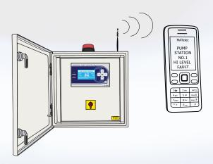
Once the signal is decoded the micro controller provides four inputs to the GSM modem which then in turn, sends SMS messages as configured.
