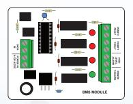
Once the signal is decoded the BMS micro controller in the Auxiliary Device provides four voltage free relay outputs for interfacing with a computer or other monitoring equipment.
