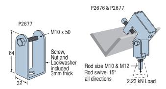
P2677 clevis hanger to be used with P2676 to provide angle adjustment and 15 degree free swing for up to M12 rod suspension. Order P2679 series swivel nuts required.
