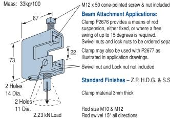
**Beam Attachment Applications:** Clamp P2676 provides a means of rod suspension, either fixed, or where a free swing of up to 15 degrees is required. Swivel nuts and lock nuts to be ordered separately.
