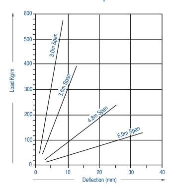
Deflections shown apply to the end-bays (ie. worst case) of a continuous ladder run. To find deflection of a single span, multiply by 2.5.
