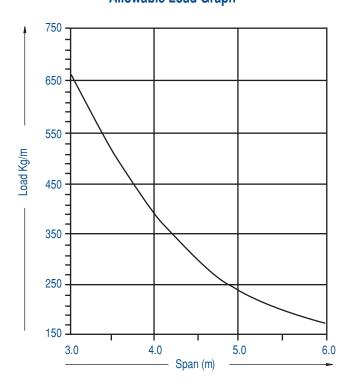
Allowable loads are determined generally in accordance with NEMA Standard VE1 and verified by testing. Safety Factor = 1.5 on collapse load for single span.
