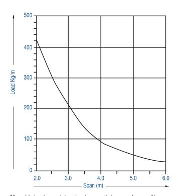
Allowable loads are determined generally in accordance with NEMA Standard VE1 and verified by testing.
