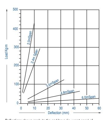
Deflections shown apply to the end-bays (ie. worst case) of a continuous ladder run. To find deflection of a single span, multiply by 2.5.
