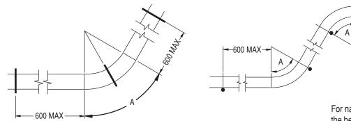
For narrower ladders and smaller angles, the bend centre support may be deleted.
