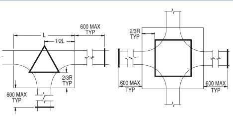
For smaller radius accessories and / or lightly loaded ladders, the support methods shown may be reduced or even eliminated.
