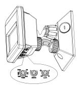
Turn LUX knob on the minimum (3). If the ambient light is more than 3LUX, the sensor would not work and the lamp stop working too. If the ambient light is less than 3LUX (darkness), the sensor would work. Under no induction signal condition, the sensor should stop working within 10sec±3sec.
